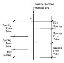
Figure 28. taggered offset fastening along marriage line
