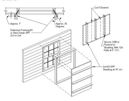
Figure 106. Wind protection shutter construction
