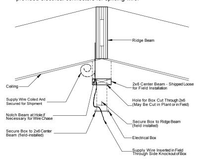
Figure 104. Wiring for a ceiling fan or chain-hung light fixture with a maximum weight of 35 lbs
