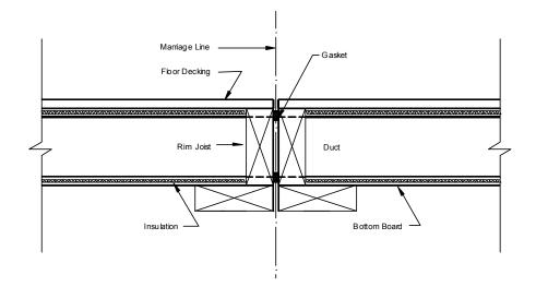
Figure 25. End wall completion
