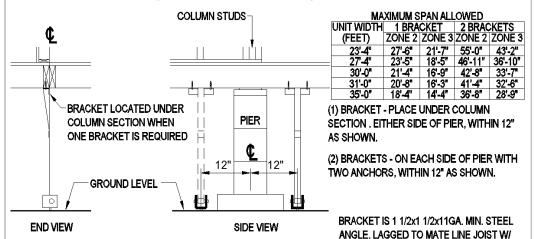
Figure 89A. Marriage line tie-down connections using steel angles. Column on one half.
