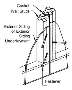
Figure 36. End wall connection toed through sheathing
