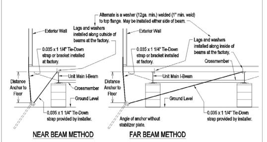
**Figure 80.** Lateral tie-down configurations.
