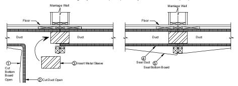
Figure 59. In-floor duct with crossover using metal sleeve
