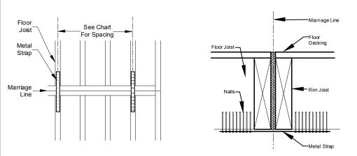
Method 2: Install horizontal fasteners through rim joist
