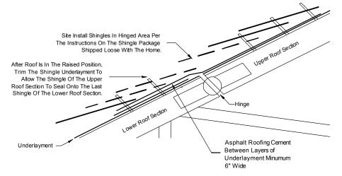
Install shingles. Install missing shingles according to the shingle manufacturer's instructions.
