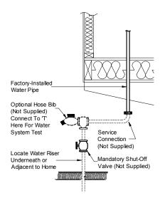
Figure 93. Water system connection
