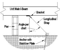
The following tables tabulate minimum number of longitudinal (frame) anchors required at each end of home.
