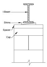
5. **Set up level.** Set up a water level with the fluid level at the desired height of the main piers. Carefully lower the side of the section down onto the leveled piers, adjusting the final height with shims.
