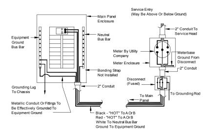
Figure 90. Electrical feeder connection when meter has a disconnect installed (typically more than 6 feet from service electric panel).
