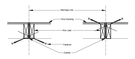
**Figure 27**. Floor connection through bottom board or floor decking
