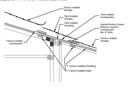
Figure 35. Triple-section roof connection Method 2
