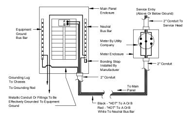
Figure 91. Meter base wiring when there is no separate disconnect installed (typically within 6 feet of service electric panel).
