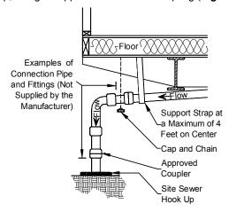
Install supports. Install permanent drain line supports at a distance of four feet o.c. or less (see Figure 70, Figure 71 and Figure 73).
