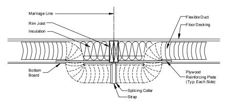
**Figure 60.** *In-floor duct with flex duct crossover under the rim joist*
