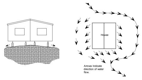
Grade the ground so that water under porches, decks, recessed entries flows away from the home. If proper grading is not possible, use other methods such as a drain tile and automatic sump pump system to remove any water that may collect under the home.
