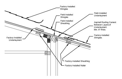
Figure 49. Triple-section roof connection Method 2
