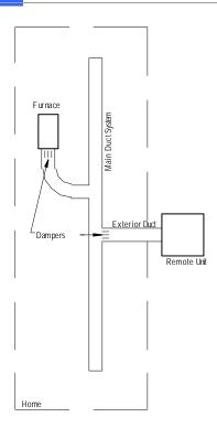
Figure 97. Remote unit damper locations
