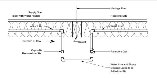
Figure 69. Water line crossover through bottom board
