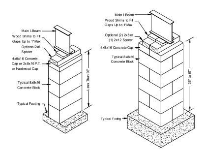
Figure 18. Frame pier construction
