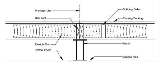
Figure 58. In-floor duct with flex duct connection though the rim joist (shown with perimeter frame system)
