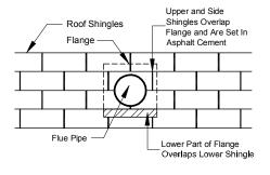
Figure 102. Roof flashing and shingle installation around chimney
