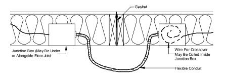
Figure 64. Under the rim joist electrical crossover connection with conduit
