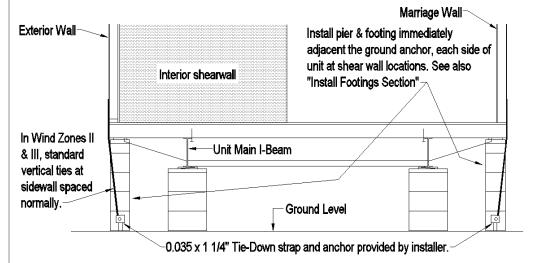
Figure 78. Shearwall Anchors.
