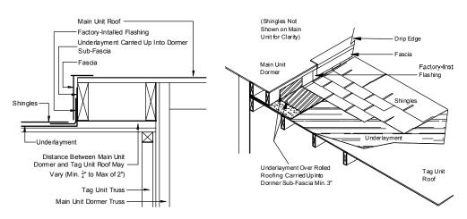
Figure 51. Tag unit roofing connection with less than two inch height difference
