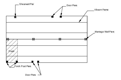
**Figure 8.** Typical point-load support locations
