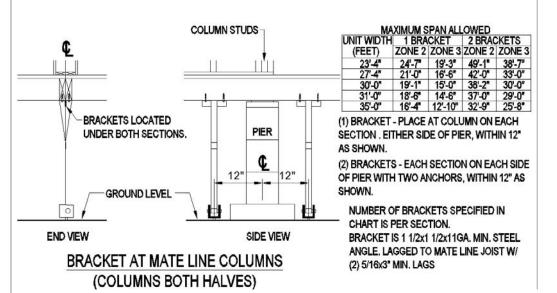
Figure 89B. Marriage line tie-down connections using steel angles. Columns on both halves.
