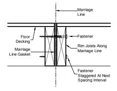
**Figure 30**. Horizontal fasteners through rim joists
