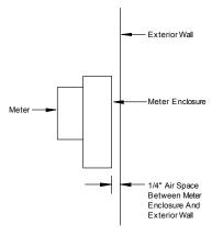
Figure 92. Meter base clearances.
