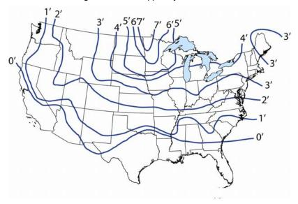
Figure 6. Average frost penetration depth (feet)
