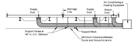
Figure 98. Ducts connecting exterior heating and/or cooling equipment to the home
