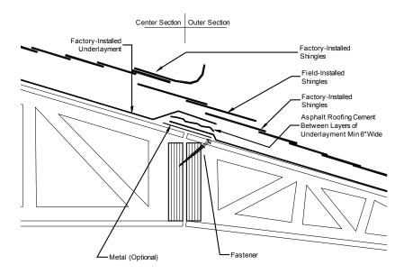
Figure 48. Triple-section roof connection Method 1
