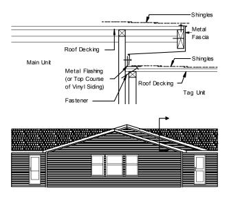
Figure 52. Tag unit offset roof connection
