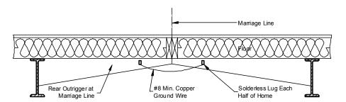
3. **Attach strap.** If ground lugs and copper wire are not provided, attach the provided four-inch bonding strap to each pair of adjacent chasses with two #8 x 3/4" self-tapping metal screws (one screw each side).
