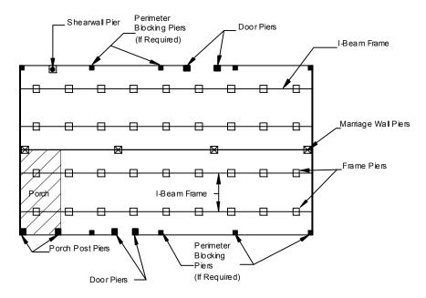
As the location and load for each support is determined, note it on the sketch. When selecting locations for supports, keep in mind that increasing the spacing between sup-
