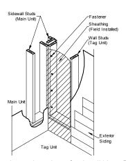
5. Connect roofs. Connect the tag unit roof to the main unit roof using #10 x 5" screws or 3/8" x 6" lag screws, toe screwed at each main unit vertical structural member (stud or truss) location. See Figure 42 for flush roof connections and Figure 43 for roof connections with an offset greater than two inches. Roof connections with an offset less than two inches do not require screws.
