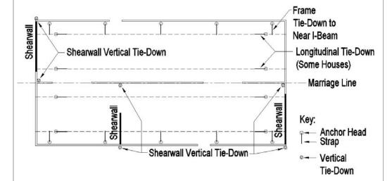
Figure 76. Typical anchor locations for a double-section home in Wind Zone I Wind Zone I Singlewide anchorage is similar using diagonal ties to near I-Beam.
