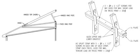
**Figure 20**. Hinged roof truss (drawing is typical, actual truss configuration may vary)
